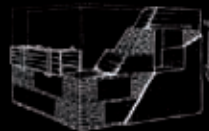
A.4.17. Rammed earth built between brick masonry pillars
